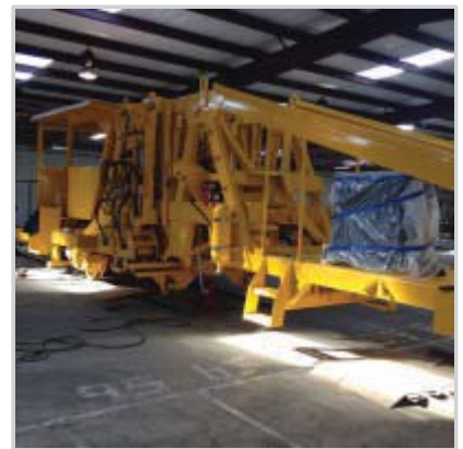
New oil cooler relocated to front deck
