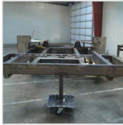
Frame extension that will convert small cab to large cab style 6700
