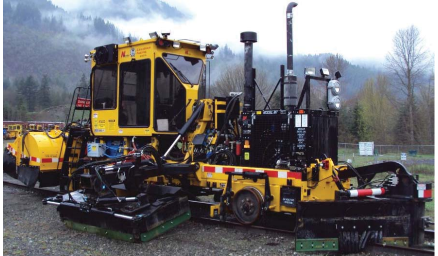
M7 - Ballast Regulator
