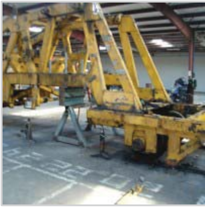
Remanufactured Harsco jackbeam ready to be installed
