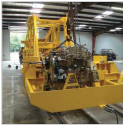
Remanufactured engine being installed
