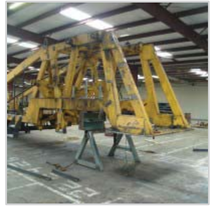
Rear platform removed and ready for frame extension to be installed
