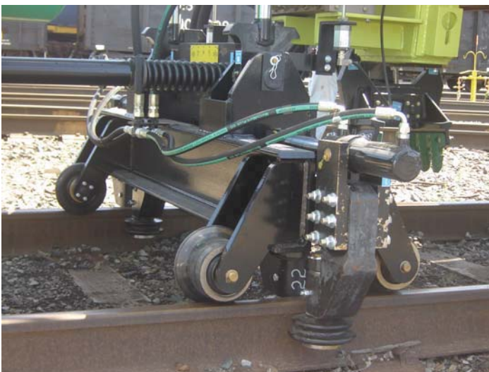
Rail jacks raise the rail while the gripper assembly inserts or removes the tie.
