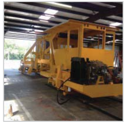
New cab, freshly painted and installed
