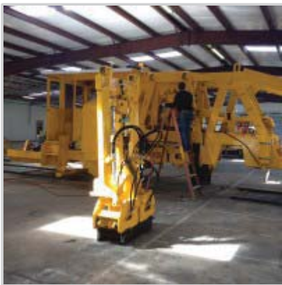
Remanufactured Harsco workheads being installed
