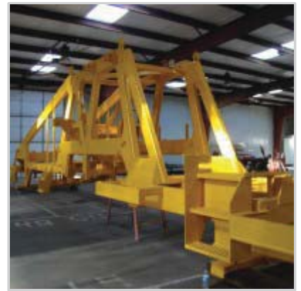
Frame extension and rear platform newly painted
