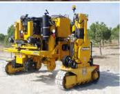
The portal is made by a main frame on which the diesel engine, the hydraulic power unit and the command console are placed.
