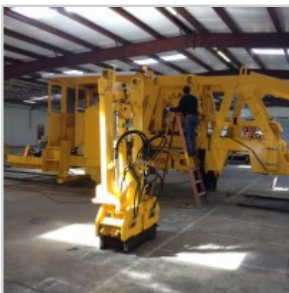
Remanufactured Harsco workheads being installed
