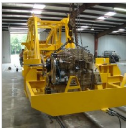
Remanufactured engine being installed
