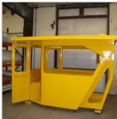
New cab built and painted, ready for install
