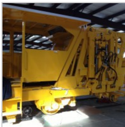
All four workheads installed
