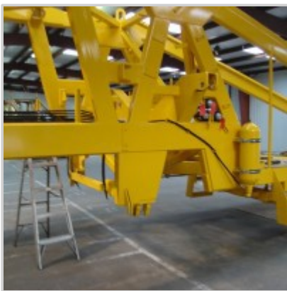
New hoses and accumulators
